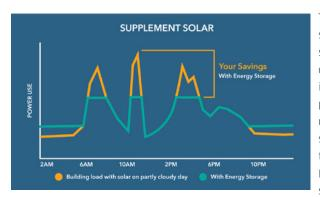
This graph depicts grid draw for a facility with solar on a cloudy day, with and without energy storage. The orange line represents the original facility load and the green line represents the new flattened load with energy storage.
